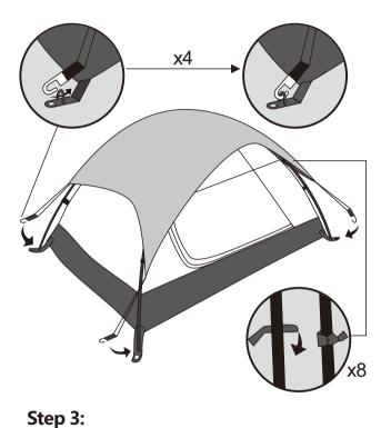
Hook the buckles of fly to the metal ring of tent in bottom corners, and tie the straps of fly to the poles..
